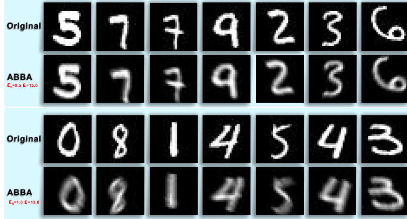
Figure VII: Visualization examples of ABBA for attacking STN-based CNN with two group hyper-parameters, i.e. , \epsilon_\theta = 0.5 , \epsilon = 15.0 and \epsilon_\theta = 1.0 , \epsilon = 15.0 .
